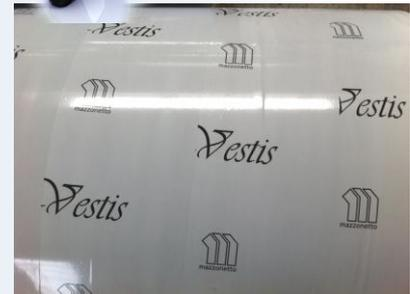
Protection film used for 0,8 and 1.00 mm thick Vestis coils.
